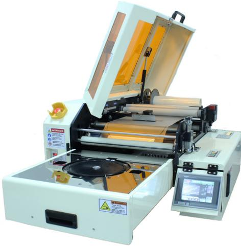
**Adjustable pinch roller pressure for easy handling of any kind of dicing tape (thickness) via air cylinder**
